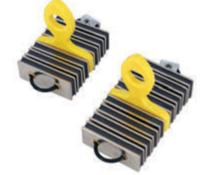
The Blanket Mate Heavy Duty Blanket Holder is an articulating magnet that safely and securely positions a rubber insulating blanket onto any metal surface. It is specifically designed to conform to curved and/or uneven surfaces. The tear drop shape end is manufactured from a unique polymer that remains strong and flexible even in cold weather.
