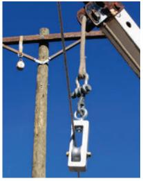
Unlike imported cast blocks, the Conductor Lift Snatch Block is USA made and machined from solid aluminum. The compact design offers a 1500 pound m a x i m u m working load yet weighs only 3 lbs.
