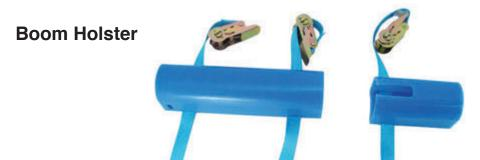
The Boom Holster is a unique two-piece hot stick holder that easily mounts on a boom. The rugged molded design is spring loaded at one end so an operator can remove and insert a hot stick with just one hand.
