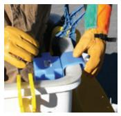
drainage holes in the base provide rain drainage to ensure the interior stays dry. The cover/base design permits bucket stick storage without the need to rotate the hot stick probe end and permits one to grab the stick body when removing so as not to extend the stick.
